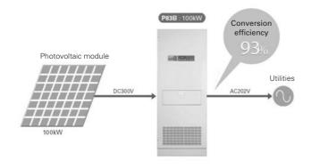
Fig. 5: Conversion efficiency for "SANUPS P83B"
